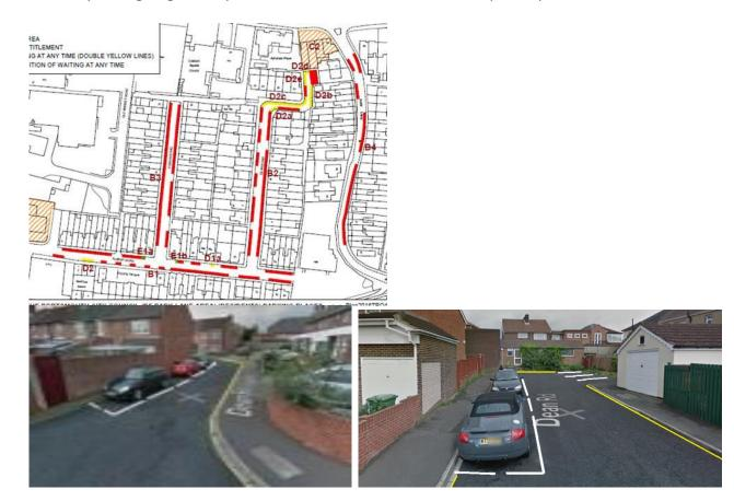
There are already double yellow lines at the northern end of Pervin Road and therefore it is not necessary to propose them there. The gaps between the parking bays shown in red on the plan above and attached indicate the dropped kerbs - parking bays cannot be marked in front of them.
